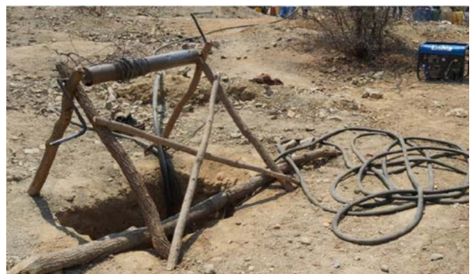
Plate 4: Makeshift winch at a pit in Kadoma
