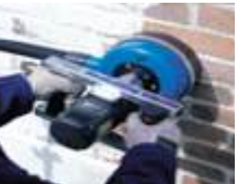
Masonry Sanding machines
